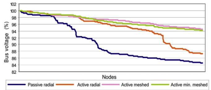
Fig. 6. Voltage profiles for the four configurations at maximum load conditions.
